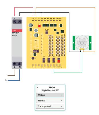
Pic. 7. Connecting an Arduino-compatible 5 V binary sensor
