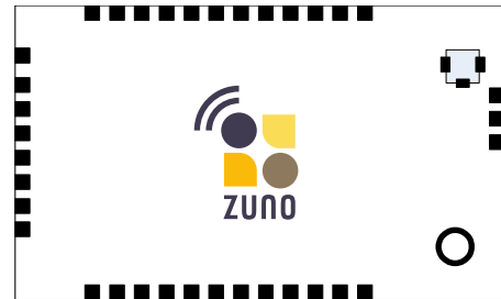
27 pins, 25 mm x 15.0 mm x 1.9 mm
