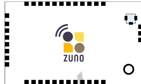
27 pins, 22.4 mm x 15.0 mm x 1.9 mm
