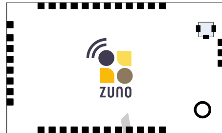
27 pins, 25 mm x 15,0 mm x 1.9 mm
